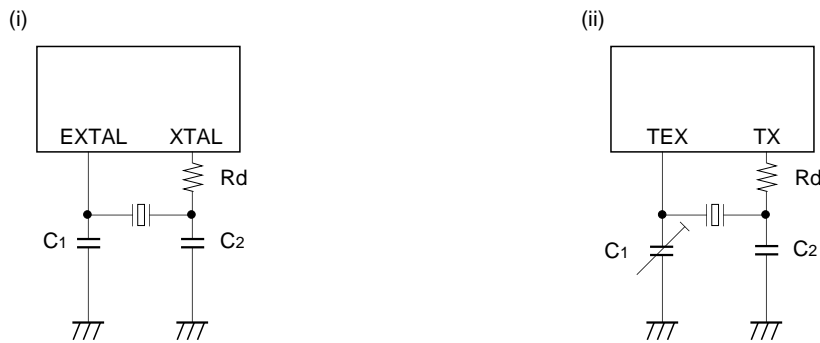
Fig. 11. SPC700 Series recommended oscillation circuit
